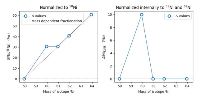
Above figure shows an example of the two normalization scenarios. On the left side is the regular -value notation as described above. As the normalization isotope, <sup>58</sup>Ni is chosen. The red, dashed line shows the internal, mass-dependent fractionation that was introduced into the system artificially. Clearly, <sup>60</sup>Ni shows some positive deviation from this line. After internal normalization, a clear excess in <sup>60</sup>Ni can be seen in the figure.
